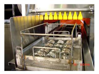
Air knives are used for spot free drying of critical components prior to the dryer
