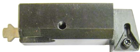
6593P Cartridge Assembly Offset Indexable Insert, Triangular, Positive Rake. Range 4.40 - 4.90" (112 - 124mm)
