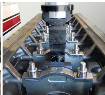
Special steel main bearing housings found in high power diesel engines such as MTU 4000 require high speed machining to obtain superior accuracy of roundness, straightness, parallelism and surface finish.
