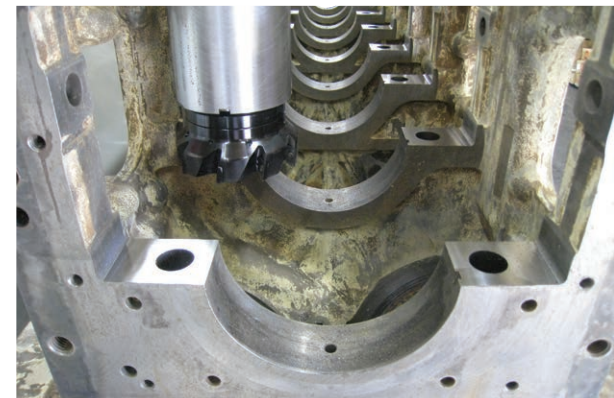
Rottler's unique right angle drives machine each bore individually and the digital display ensures perfect accuracy and alignment.
