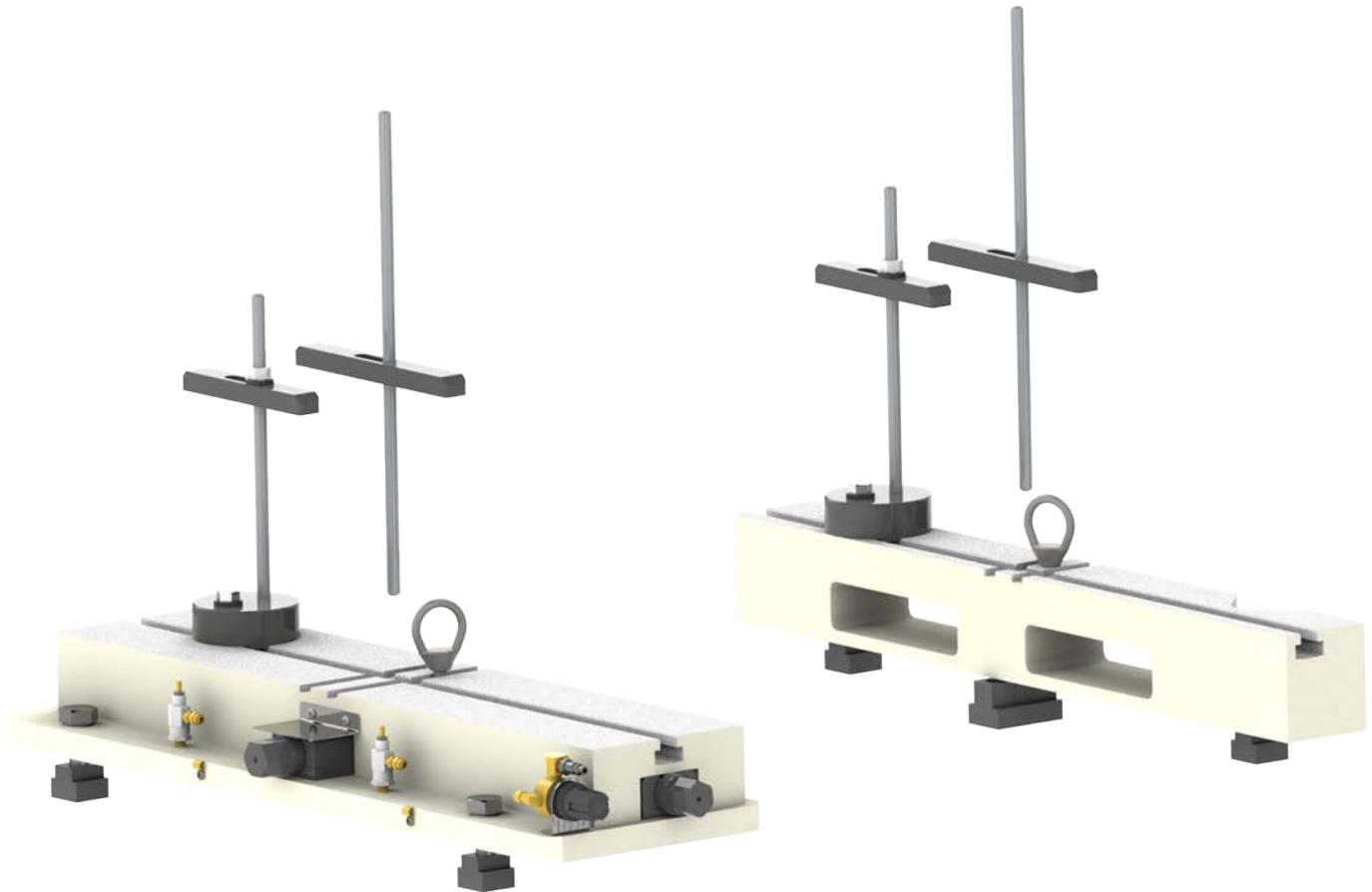
**6823B 120 Degree V Block Supports for Large 120 Degree V Blocks**
