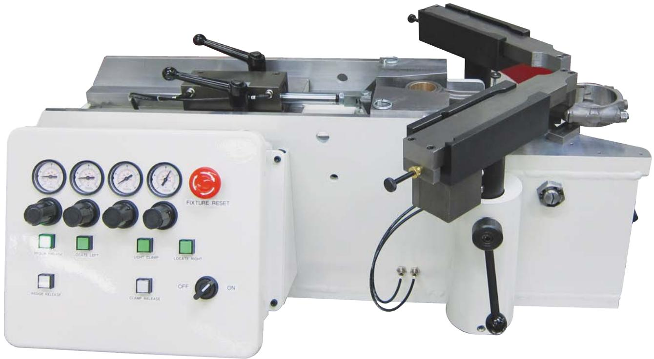
**Fixturing & Tooling for Machining Large Engine & Compressor Connecting Rods****650-3-64 Rottler Precision Connecting Rod Fixturing System**
