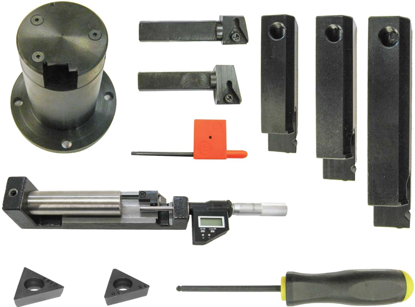
**6519N Heavy Duty Line Bore Cutterhead Assembly**
