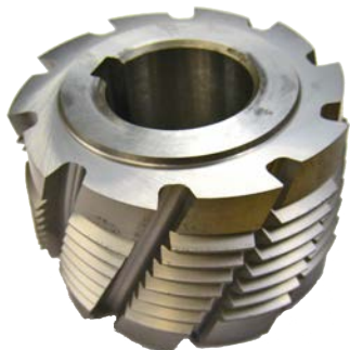
6868 Six pitcher cutter used on the VHP rod and some CGF rods
