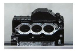
Marine Outboard, Snowmobile, Motorcycle and other similar cylinders can be easily mounted and rolled over for precision blind hole honing.
